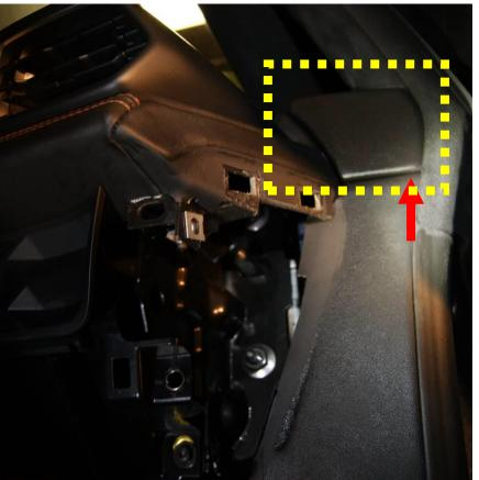
(6) With the 6 screws removed, now you can pull up on the top molding to release the "Internal Side Member".
