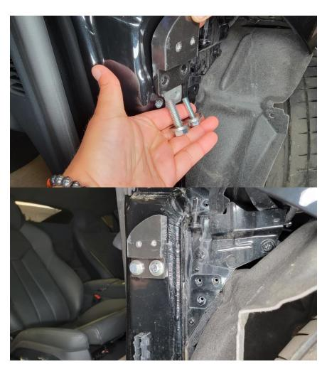
To install the hinge you will also need to install the bottom spacer as shown. The spacer uses the same bolts as the hinge. Use the M8-1.25 X 60MM + washer on the hole nearest of the wheel and the 7/16-14 X 2-1/4 HEX HD on the 7/16-14 Threaded Inserts (the hole nearest the back of the car as shown).
