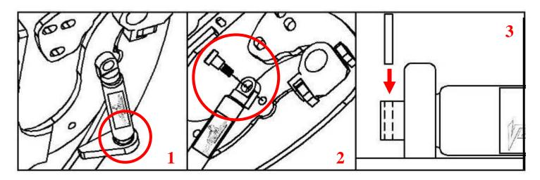
Hint\* (You will need a helper to raise the door). (Slip the spherical rod mount into the spherical ball bearing (1). Using a 1/4 Allen wrench, tighten the screw into the swing arm (2). After the shock is installed secure it by installing the pin in the bottom shock end (3).
