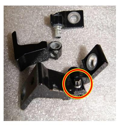
Once the door has been removed you can now remove the factory door hinge from the body. Remove the one bolt closest to the front of the car. To remove the bolt towards the back of the car you will have to grab the hinge and turn it counterclockwise as shown below.
