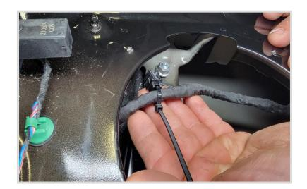
Pull the wire boot from the front of the door. Break the bottom of the wire harness to remove the factory wire harness connector cover. As shown.
