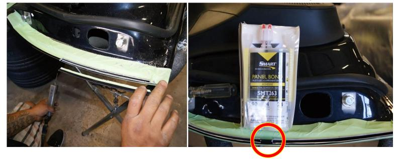
VERY IMPORTANT, make sure to leave a piece of the front door to keep the original door gap as shown above.
