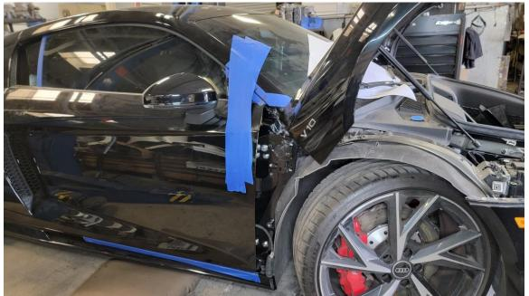
This is a VERY important step. It will make the door alignment easier during the installation. Use a spacer at the back of the door to keep the original door gap. You can use a paint stick or something similar.
