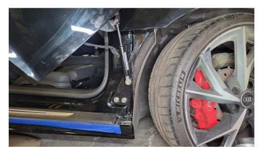
Make sure to install the door on the factory location using the marks and measurements taken before the door was removed.
