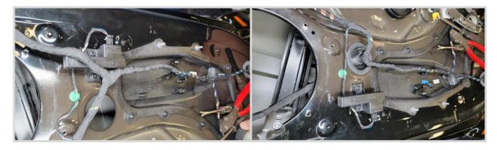
Use the factory wire clips to secure the wires to the door.
