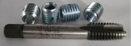
We use a 17/32 drill to enlarge the factory hole to accept the Drill tap.
