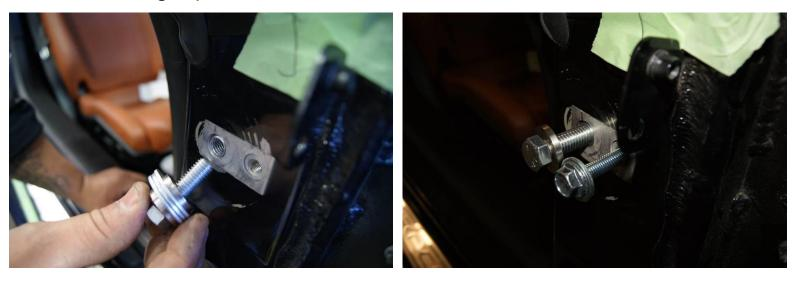
The new VDI kit opens the door on the outside of the fender.
