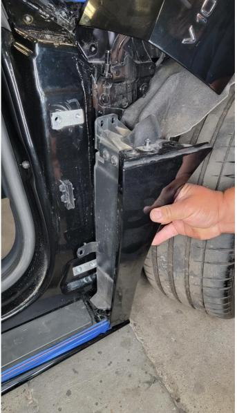
After removing the fender, remove the plastic trim for the fender as shown below.
