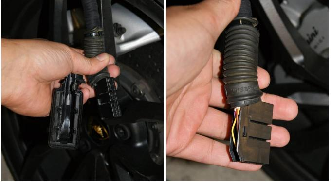
Plug the door wire harness to the body wire harness and put it inside the body.
