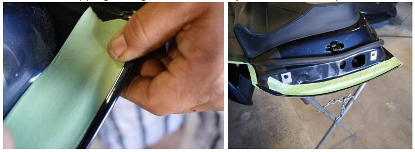
Cut the front lip of the door as shown. You will need to leave a small piece of material in the middle so that the door keeps its original gap.
