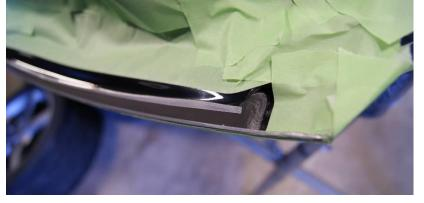
Once the panel bond has dried cut off the remaining piece of the door and fill it with Panel Bond. Once dried use a grinder to smooth out the Panel Bond to get it ready for painting.
