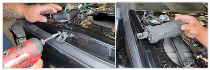
Remove the door wire boot as shown. It has blue around it carefully tear it off so that you can slide it towards the front of the door as shown.
