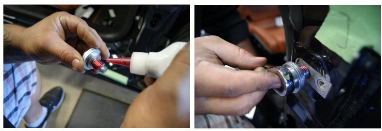
Once the tread insert has been secured, remove the bolt and clean the extra "Loctite".
