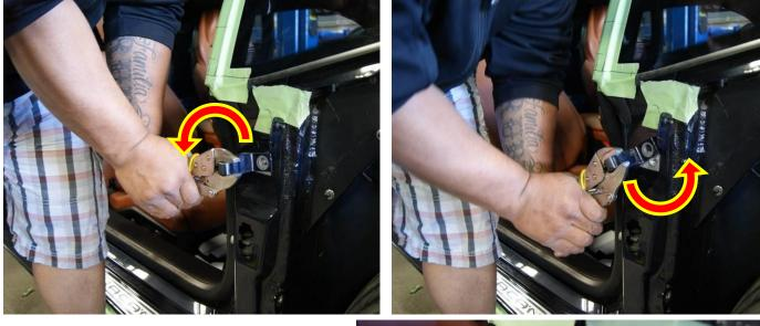
Once the factory hinge has been removed from the body, you will see a bolt sticking out, you will have to remove the inside dash molding to remove the bolt.
