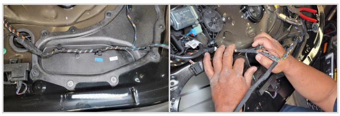
With the factory wire fully covered push the wire boot back into the door hole as shown.
