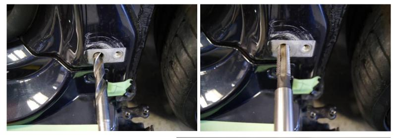
To install the new hinge you will need to use 7/16-14 "Thread Insert". You will also receive a 5/8-11 Tap. The Thread Inserts and the Tap are included with the kit.
